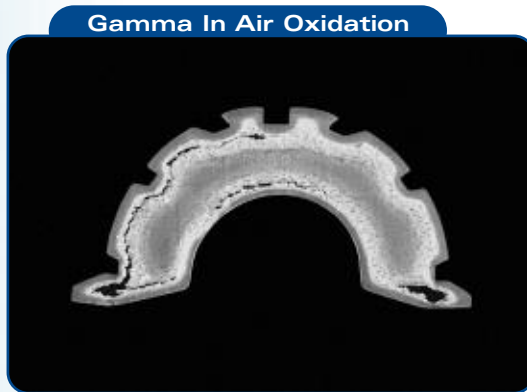
Shelf-aged, gamma in air-sterilized polyethylene demonstrating significant oxidation.
